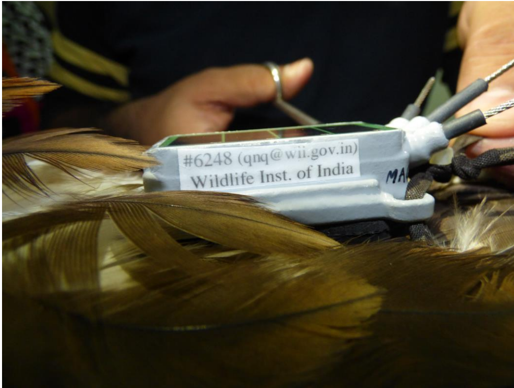
Fig 8. Black Kite Project Research team affixing a GSM tag to a Black -eared Kite ( Milvus migrans lineatus ). The tag in the image has a solar panel on the top, and is affixed on the birds using a tubular teflon harness.
