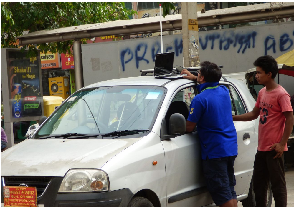
Fig 14. The research team in the above image has set up a two-way communication with a GPS tag affixed on a kite of the resident subspecies Milvus migrans govinda . The telemetry data from the transmitter can be read using a hand-held, portable base station. The same base station is used to re-configure the tag using a laptop and an omni antenna fitted on the roof of the vehicle.
